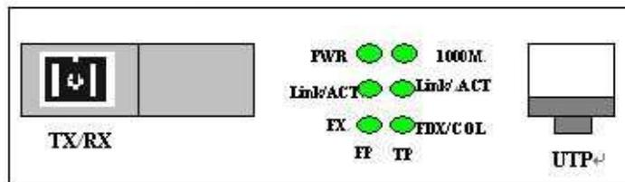
Table 2 : Front panel for dual fiber media converter
